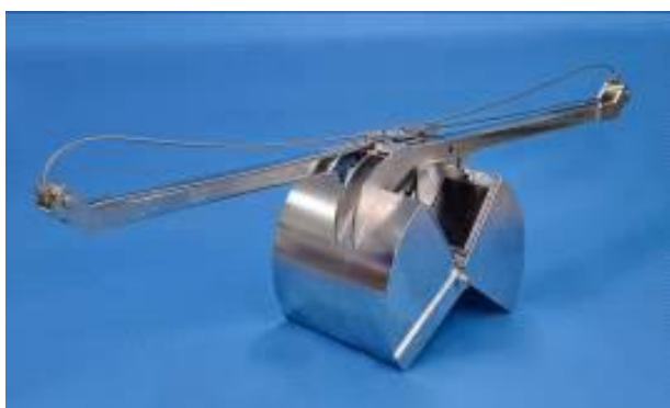
Figure 3: Sediment sampling device
