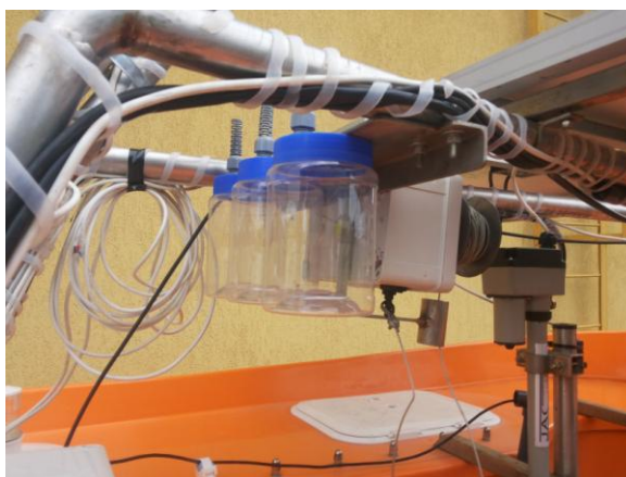
Figure 2: Water sampling device (3 bottles)
